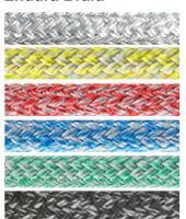
Endura Braid™ features a specially engineered 12-strand Dyneema® SK78 core, with Marine-Tech coating, and a 24-carrier braided polyester cover.
