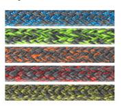
Poly Tec uses the same high-strength lowweight Dyneema® core as Endura Braid while adding an extra durable cover made from a blend of Technora and Polyester fibers. Poly Tec offers excellent abrasion and cut resistance, heat dissipation, and a level of grip that other high performance ropes don't offer. Use for applications that require a low stretch, low creep, and extra-grippy line such as halyards, sheets and control lines.
