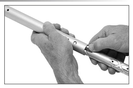
**Loading Injector with Adhesive**
