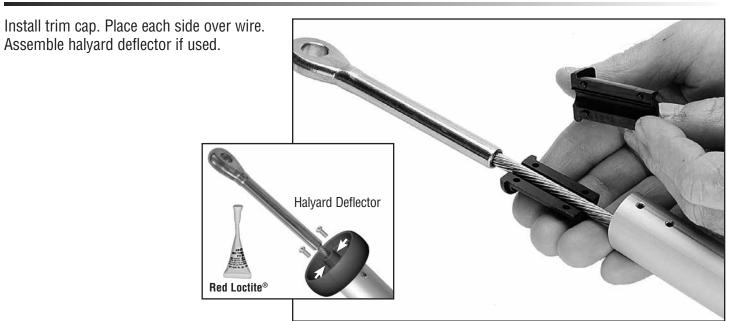
Push trim cap into foil to start, then tap in using hammer.
