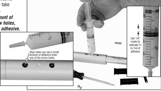
Tighten screws into connector holes. Make sure a drop of red Loctite® entered each screw hole. If not, apply to screw.
