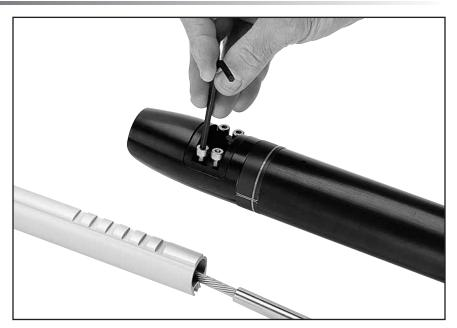
Slide drum assembly onto foils.
