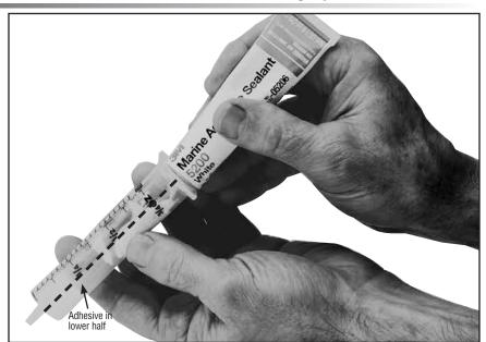
Start plunger into injector and immediately hold upright so plunger is down and applicator tip is up.
