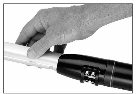
Slide halyard swivel above feeder. Place feeder in foil recess. Push screw down so tab catches under foil. Tighten screw.
