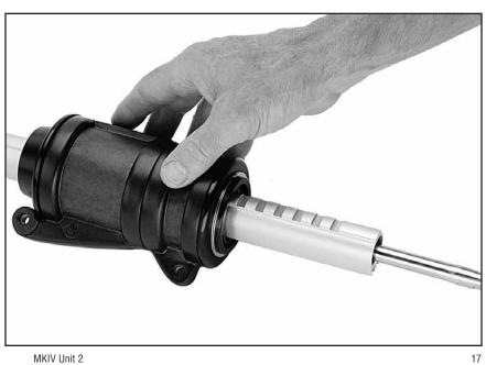
Loosen foil clamp screws at top of drum assembly.
