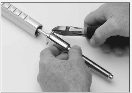
Assemble turnbuckle and attach Harken toggle.
