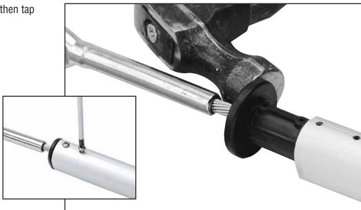
Place halves of plastic bushings on stay so hooked part of longer section faces out.
